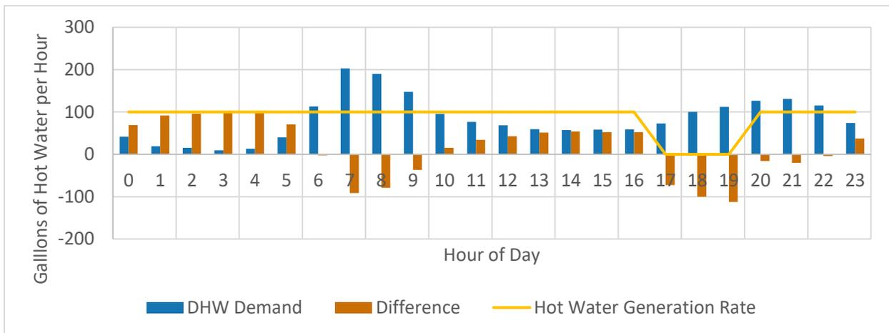
**Figure 11. A load shift scenario where the systems is HPWH is excluded from 1700 to 2000.**
