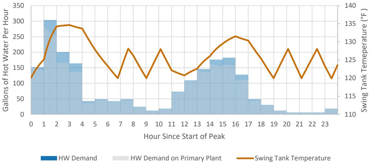
**Figure 9. Swing tank simulation plot.**
