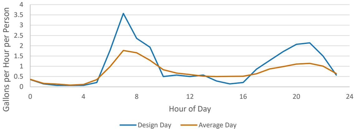
**Figure 5. Measured Load Shapes from Ecotope Buildings.**
