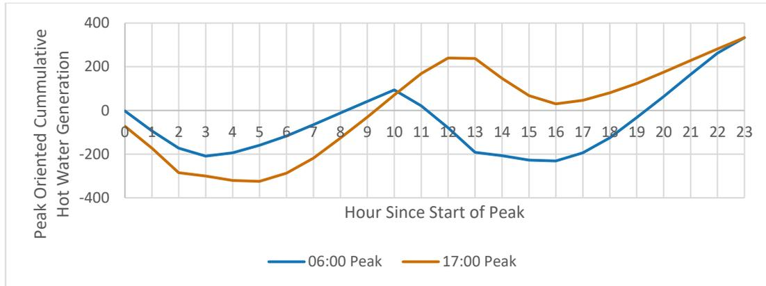
**Figure 12. The cumulative supply after peak events for a load shift scenario.**
